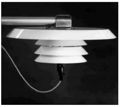
The Model 073B Naturally Aspirated Radiation Shield is used in remote areas, where power is not available.
