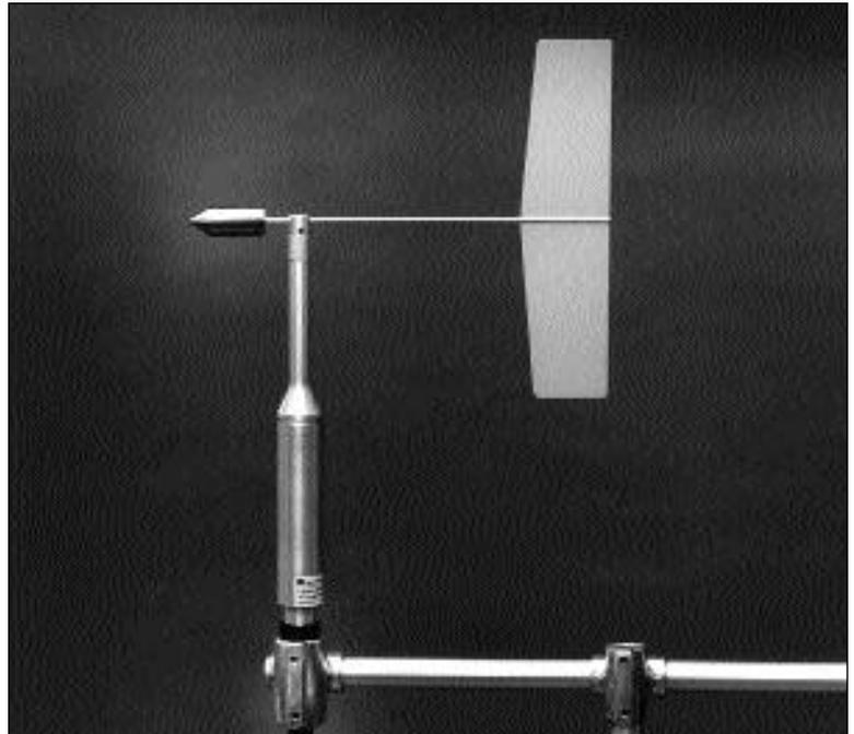
The Model 020C is useful when a low starting threshold, a high damping ratio or short delay distance is required.
